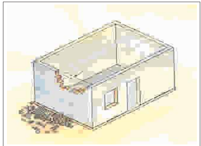
Wall with small portion at top having collapsed
